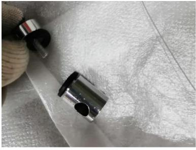
4. There are 4 holes on the windshield, assembling the two parts as follow for each hole, the shorter one at the front side of the scooter. (windshield)
