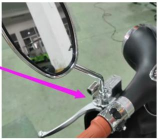
2. Then find this poles, and nuts (two sets), and another nut, then insert in the before part, both side do like this.
