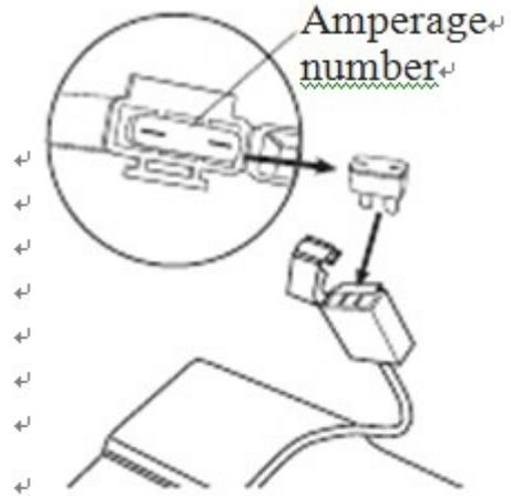
Remove the fuse and replace with a new one of equal amperage. Requires 30 amp fuse. Close the fuse cover and reattach the battery cover.
