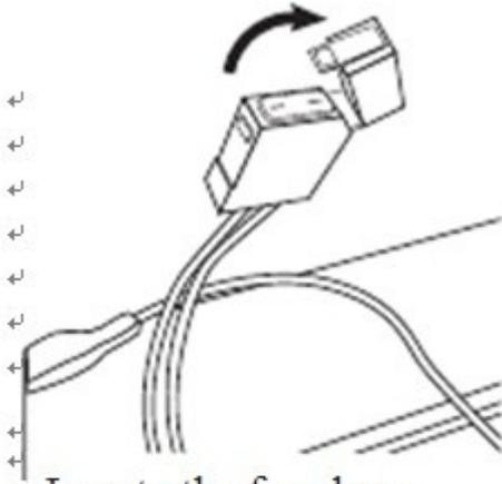
Locate the fuse box attached to the batteries. Open the fuse cover to expose the fuse.
