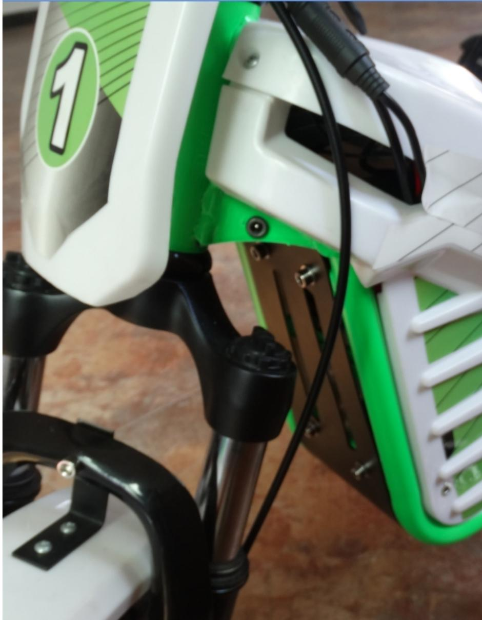
The charge port on this vehicle is on the left side of frame, on top of the front shock, and behind the number plate ( see above pictures)
