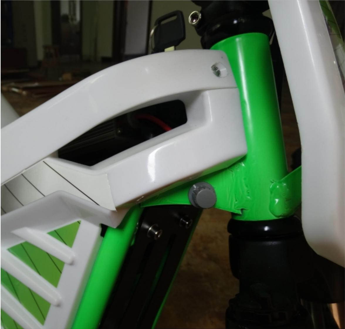
The speed limit switch is located the right side of front fork behind the front number plate.
