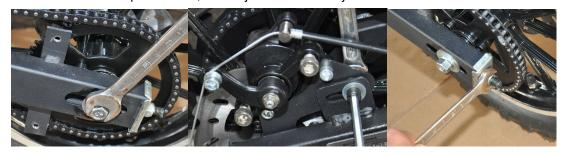
**Step 3:** The chain tension is in good condition while the gap is about 5mm between chain to lowest parts of swing arm. Lock all the nuts and screws, check the wheel alignment and then re-attach the chain cover.
