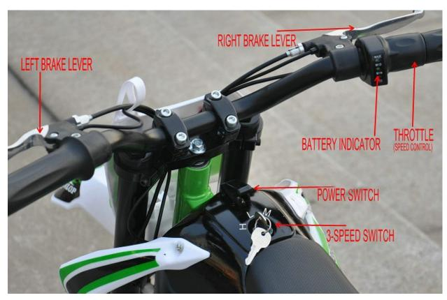
**BATTERY INDICATOR Note:** STOP using the bike and charge the battery once the indicator turns into red and yellow light only.
