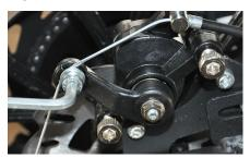
If the brake has too much slack, loosen the rear anchor bolt with a L-wrench and pull the brake wire tighter.
