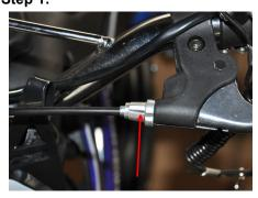
To adjust the brake tension, thread the brake lever adjuster in or out 1/4 or 1/2 turn until the required brake adjustments are attained.
