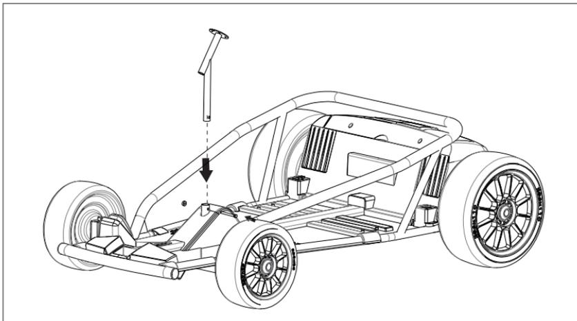
②. Insert the steering axle from the bottom to the car body and steering axle holder, until the top of the steering axle extends out the steering axle holder.
