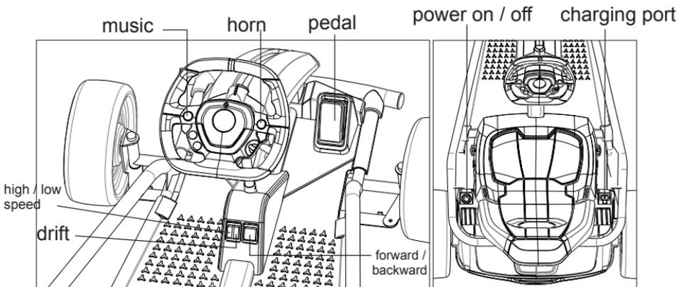
There is a “drift / driving” mode switch on the car, press the drift switch up, so the drift function can be used.
